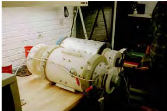
EMA4 and EMA5 Motors at the time of recovery in 2000 With external Control Commutators mounted on the right
