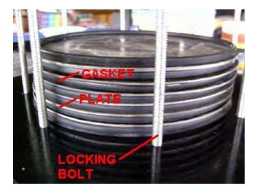
To make sure that the locking bolts do not short-circuit the plates, they are fitted with 3/8" (9 mm) outer diameter / 1/4" (6 mm) inner diameter rubber fuel-hose material.
