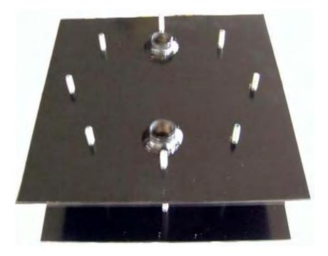
There are two strong A36 steel alloy end plates which act as clamps to lock the remaining plates in position as well as acting as electrodes. A ring of eight cadmium plated steel bolts are used to lock the unit together and these bolts also keep in position, a set of circular plates and O-ring gaskets (McMaster-Carr, Part Number - 9557K338, made of EPDM - Ethylene Propylene, Outer diameter 6.4" or 162 mm) as shown here:
